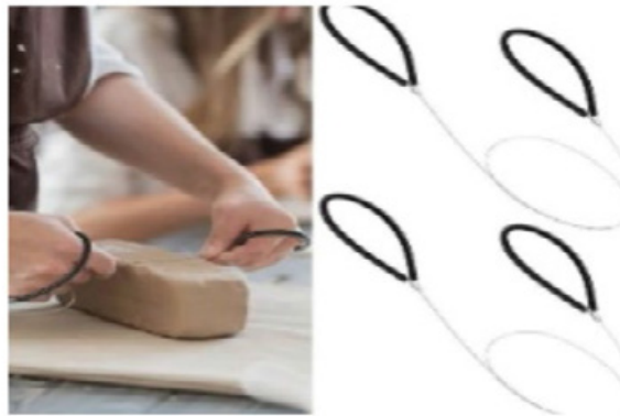
Figure 8: A piece of cloth and a metal wire for cutting clay slices, shape.
